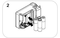
Remove the batteries from the housing. Replace with four premium alkaline AA batteries. Dispose of or recycle used batteries according to local regulations.
