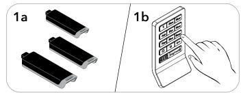
Collect all remaining and any new Manager Keys. Go to any lock operated by the Manager Keys. Press C 0 5 5 0 .
