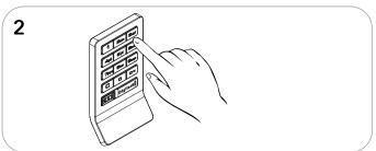
Enter the number of hours from 1 - 9 9 then press 0m. Two sets of two-tone beeps will be heard and the LED will turn off. For example: Press 8 om to set the lock to auto unlock after 8 hours.
